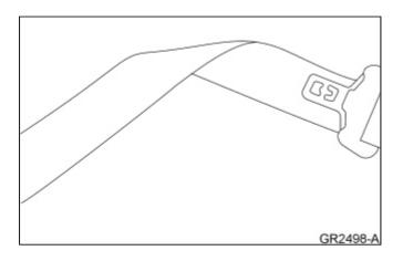
2. Pull the safety belt tongue over the fold in the safety belt.
